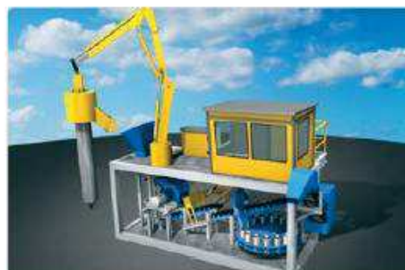
Auger Sampler Sampling equipment for sample retrieving from coal trucks and rail cars
